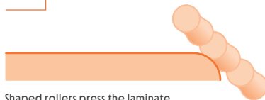
Shaped rollers press the laminate to the edge of the substrate
