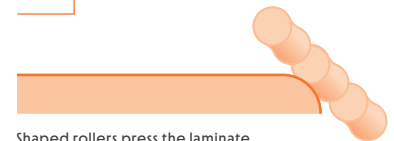
Shaped rollers press the laminate to the edge of the substrate
